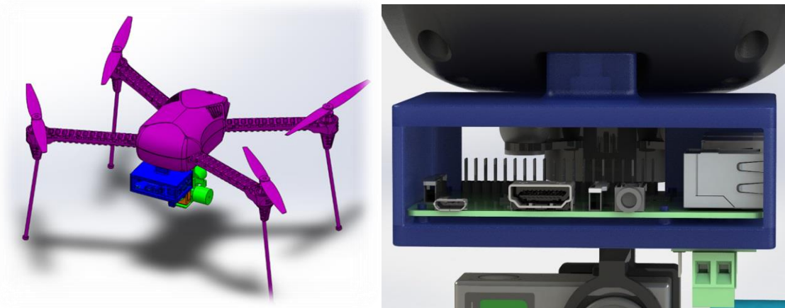
Figure 7. (Left) System View with Raspberry Pi and Mount Highlighted in Blue and (Right) a Close-up Rendering of the Raspberry Pi in its Mount
